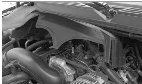
3. Lift up on the front of the engine cover to disengage from the mounting grommets. Then pull forward and remove the engine cover from the engine as shown.
