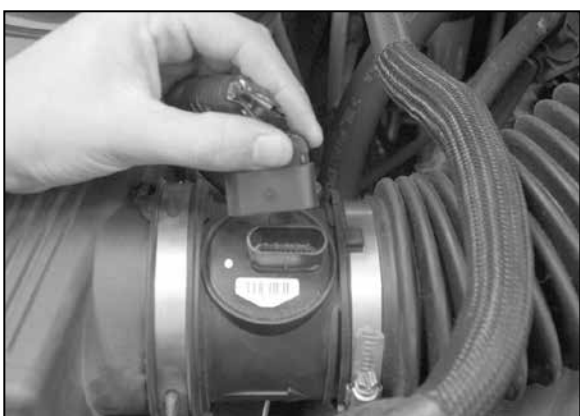
2. Disconnect the mass air sensor electrical connection.
